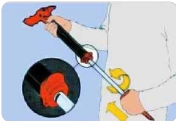
3. Push back to red line. Twist half a turn.
