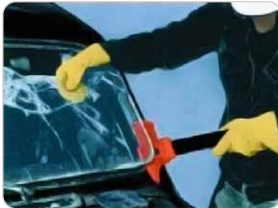
5. Remove windscreen with the breaking edge or with chisel.
