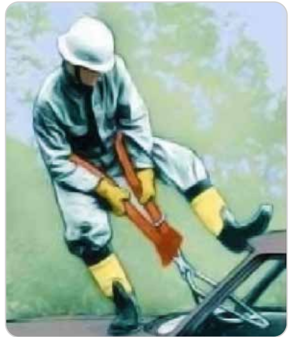
2. Bend legs and tighten belt. Pull by straightening legs.
