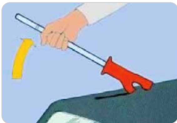
7. Rapid cutting in thin sheet metal.
