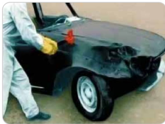
2. Cut the mudguard - use the pike.
