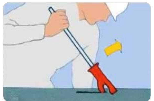
8. Only claw part in thin metal - car roofs, driver cabins etc.
