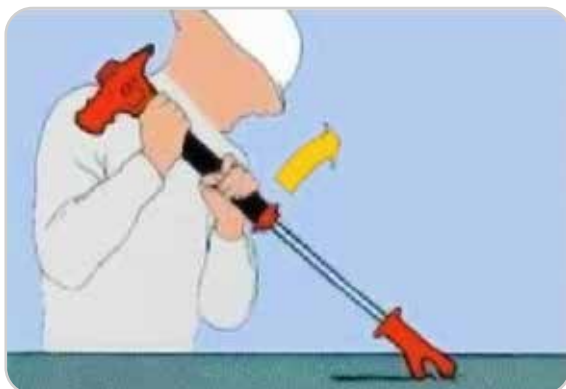
7. Long leverage in thick sheet metal (2-3 mm).
