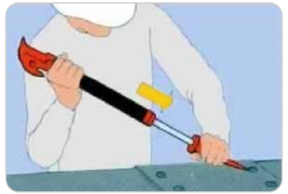
2. Cutting off rivet- and boltheads.
