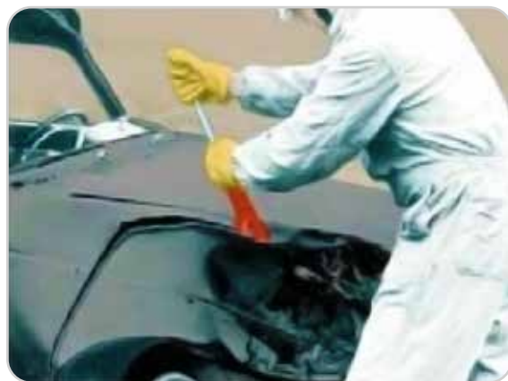
4. Cut the mudguard - use the claw part.
