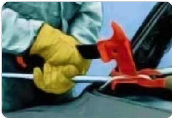
3. Cut cables while holding them with claw apart.
