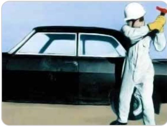
1. Release tension by hitting. Use curved side of axe part.
