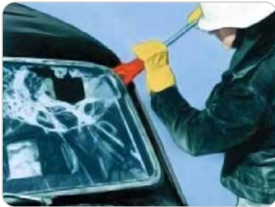
3. Loosen rubber insert with chisel.
