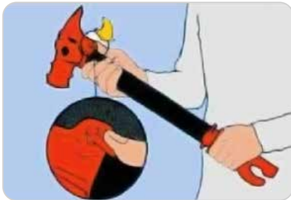
1. Unlatch locking device.
