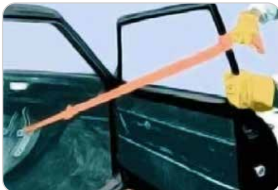
4. Strap attached to the door using the door as leverage.
