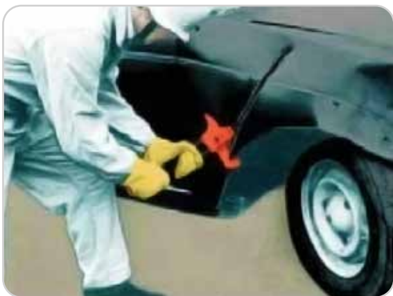
3. Cut the mudguard - use the edge.
