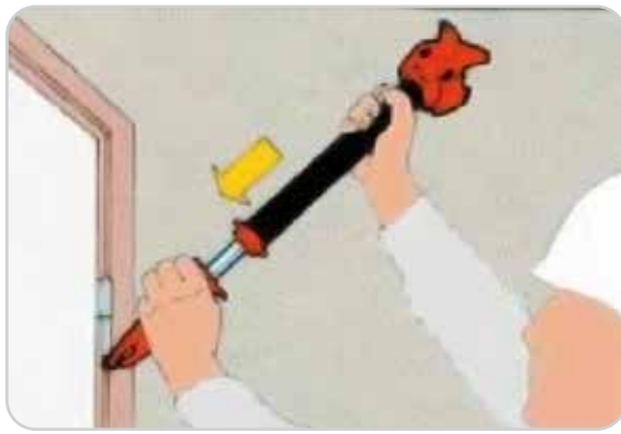
1. Pushing out pins and bolts.
