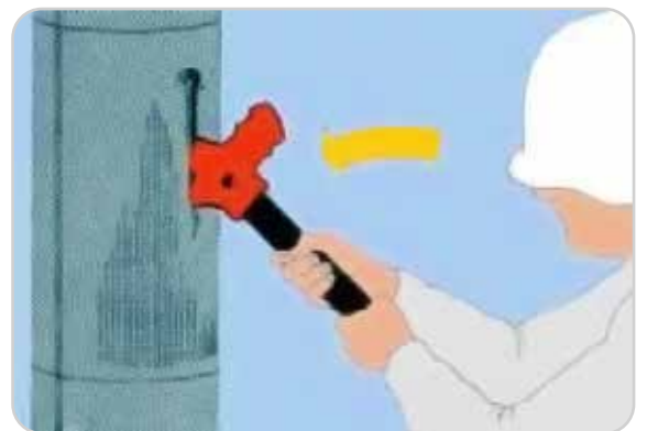
8. Thin isolating sheet metal - use axe-pick.
