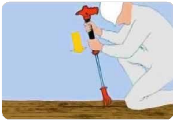
1. Pierce floor with pumping motion.
