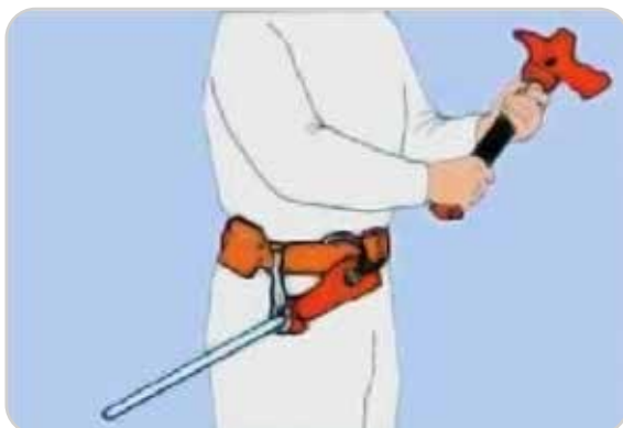
7. Claw part attached to hook and D-ring.
