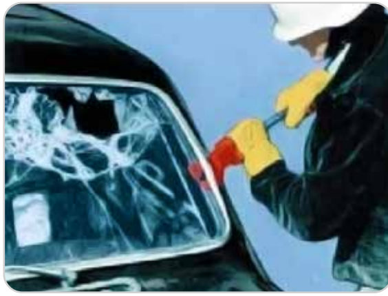
1. Loosen chrome strip with chisel or axe-pick.
