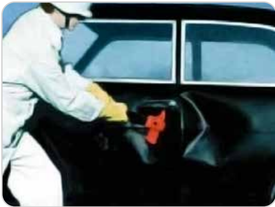
3. Hit on both sides of the lock.
